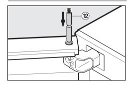
■ Place hinge pin ⑫ into the bearing block from above.
